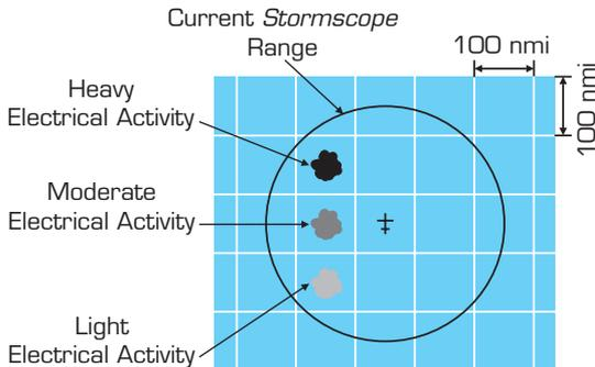
Figure 4-1. Airspace Diagram
